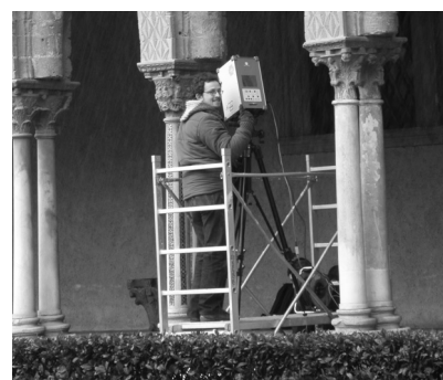
Figure 3: The acquisition setup adopted to scan the capitals.
