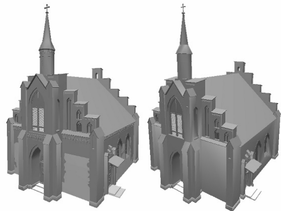
Figure 10: 3D volume model of church Raduhn in comparison: photogrammetry (left) vs. laser scanning (right)
