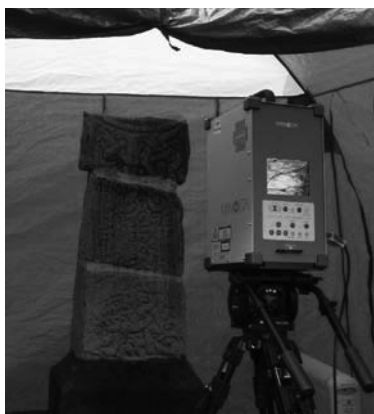
Figure 1: Scanning an Anglo-Saxon Cross using a Minolta VL-900.
