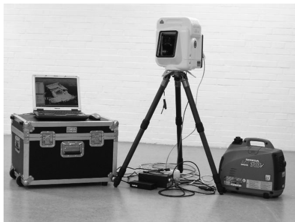
Figure 3: Terrestrial 3D laser scanning system Mensi GS100 at HafenCity University Hamburg
