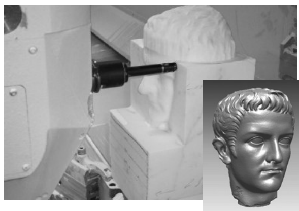
Figure 4: CNC machining a new block of Carrara marble and a screenshot of the data (insert).
