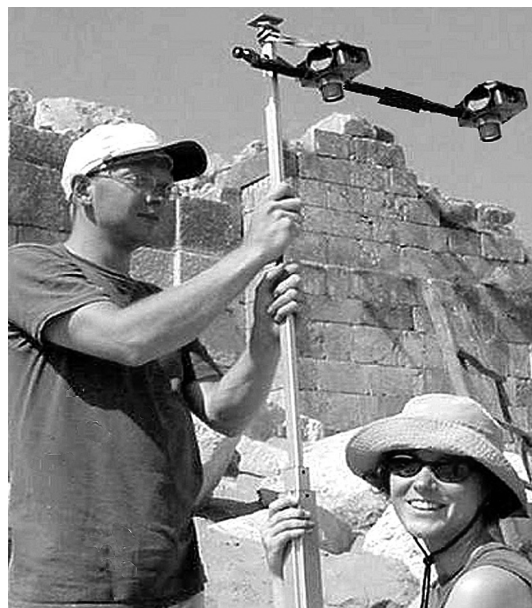
Figure 9: The digital 3D-Rod-Camera Lite with remote control doubtless becomes the most common sensor for extremely close range aerial photography (experimental study)
