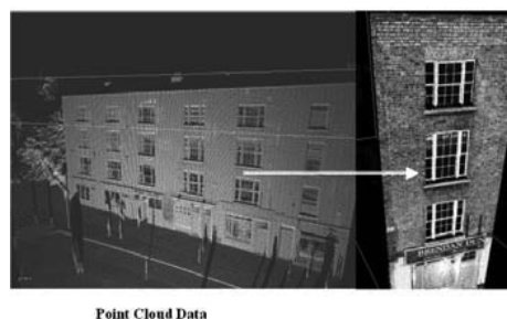
Figure 2: Point Cloud of Capel Street 18 th century Façade
